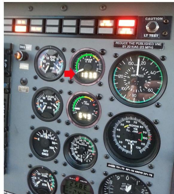
In an OGE hover, even a slight descent can lead to a big power rise. As the helicopter descends vertically at one or two hundred feet per minute, the power needed to keep from accelerating downward rises by perhaps two to five percent according to Nick Lappos, a former Sikorsky test pilot and engineer. If the descent continues unchecked, without accelerating forward to obtain some effective translational lift, the vortices created by the rotor will increase and could lead to full VRS.
