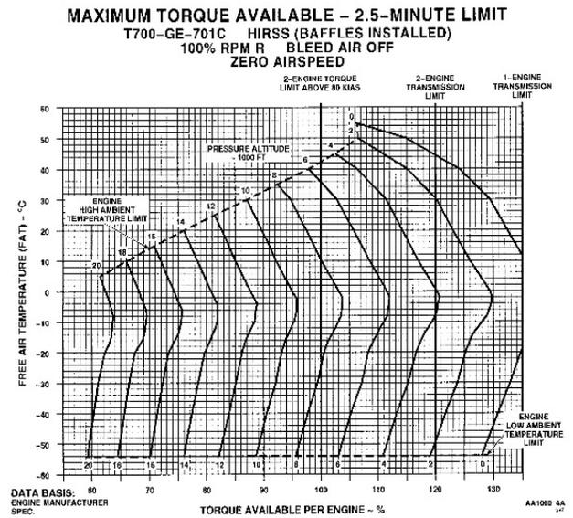
Figure 7A-4. Maximum Torque Available (Sheet 1 of 3)
